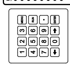
Note : For Operating Mode and Pump Setup, press **[MENU]** followed by **[ENTER]** to scroll through Menus. Use **[UP/DOWN]** to access Code.
